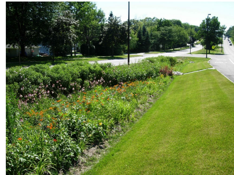
Figure 42: Bioswales can passively manage onsite stormwater in a natural and aesthetically pleasing way
